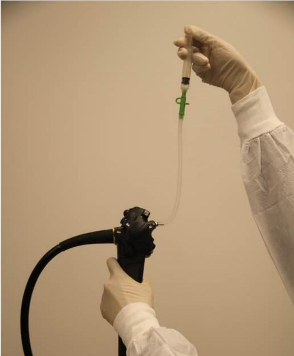
**Keeping duodenoscope vertical when flushing fluids through channels to distal end (A5.3.5.6)**
