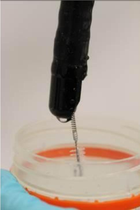
Sample container with liquid extract and swab and brush heads (prior to A5.3.6)
